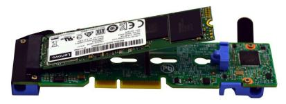
Figure 1. Dual M.2 Adapter and a 128 GB M.2 drive
